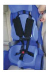
Place your knee in the MPS, bearing weight on the seat, to make it fit snuggly to your vehicle.
