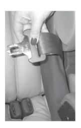
Thread the Lap/Shoulder Belt from the back to the front through the opposite slot in the seat shell located between the seat and back cushions
