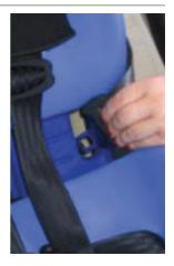
Thread the Lap/Shoulder Belt from the front to the back through the slot in the seat shell located between the seat and back cushions.
