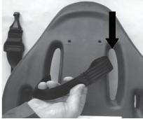
Thread loop end of Tether Strap down through right shoulder slot.
