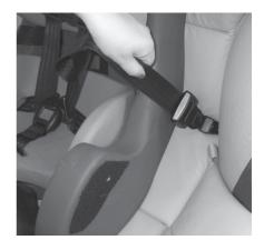
Place your knee in the MPS, bearing weight on the seat, to make it fit snuggly to your vehicle. Pull tightly until slack is removed from LATCH adjuster strap.
