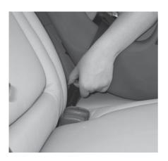
Snap both LATCH belt buckle into corresponding LATCH anchors until you hear an audible "Click" for each buckle.
