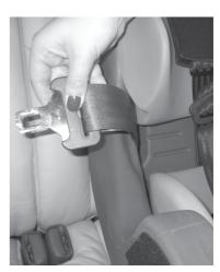
Thread the Aircraft Lap Belt from the back to the front through the opposite slot in the seat shell located between the seat and back cushions.
