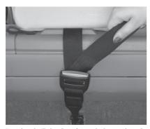
Now that the Tether Strap is attached correctly, verify tha the Lap / Shoulder belt is secured and tight.
