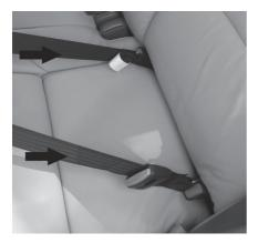
Verify that your vehicle is equipped with LATCH anchors Consult your vehicle manual to locate the exact position of the LATCH anchors.
