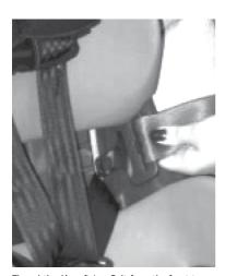
Thread the Aircraft Lap Belt from the front to the back through the slot in the seat shell located between the seat and back cushions.
