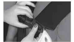
To disengage the Chest Clip, to remove your child after you are finished using the restraint, depress the two black prongs in the center of the Chest Clip and pull the two halves apart.
