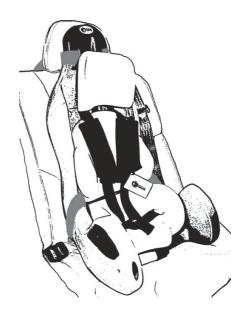
Install the MPS with the LATCH Belt & top Tether Strap.
