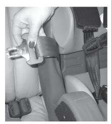
Thread the Lap Belt across the back of the seat shell.
